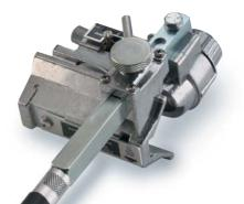
**1542-2AS - Combination Stripper** With Wedge Blade installed, spare Straight Blade
